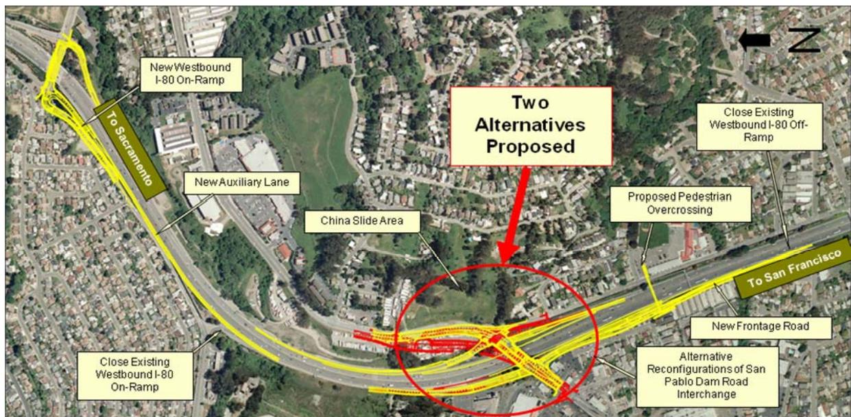
The “Lanes Added” build alternative (Alt-1) would replace the existing four-lane San Pablo Dam Road overcrossing with a new wider six-lane bridge with shoulders and sidewalks on the same alignment as the existing overcrossing (Figure A).
